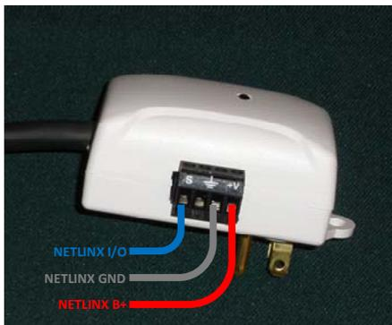
EXAMPLE USING NETLIX PWR SUPPLY
