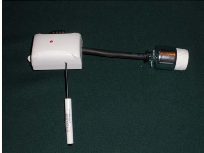
1. Please note that the adjustment potentiometer on the left side of the unit (opposite side from the Phoenix connector) has only 340° of motion. Do not try to turn it past its stops. Also, please read notes below before attempting the adjustment process.
