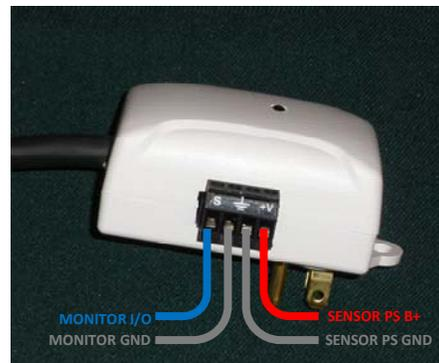
EXAMPLE USING SEPARATE PWR SUPPLIES
