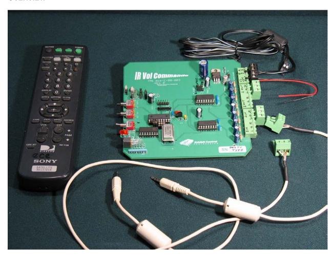
The IR Vol Commando is an infrared controllable line level volume controller. It is capable of controlling two separate unbalanced stereo channel pairs for a total of four channels of volume. It is can be controlled via an IR hand-held remote. But, its real purpose is to provide a method for controlling a conference room audio-video system's program and microphone volumes via any number of integrated IR control systems on the market today.
