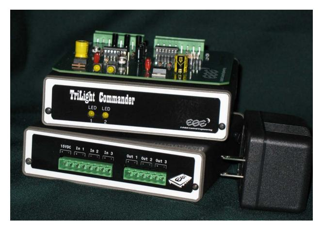
The TriLight Commander provides an interface between three switch type inputs (dry contact closure or TTL voltage) to three voltage controlled dimmer circuits (0-10vdc). Control of the following characteristics can be set for each circuit:
